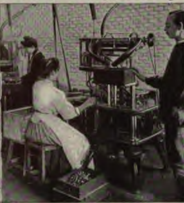
3. Charging the metal cartridges. The machine puts in the cap, measures the powder, and fastens the ball in the shell.
